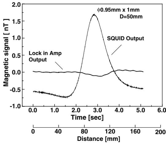
**Figure 5.** Time domain signal traces for a stainless steel chip. The SQUID output signal shows a large peak: as high as 2.7 nT (peak to peak). The lock-in amplifier output shows a small bump at around the same time.
