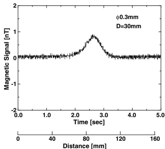
**Figure 9.** The time signal trace of a 0.3 mm stainless steel ball at 30 mm from the sensor. A peak of 0.9 nT can be clearly observed.
