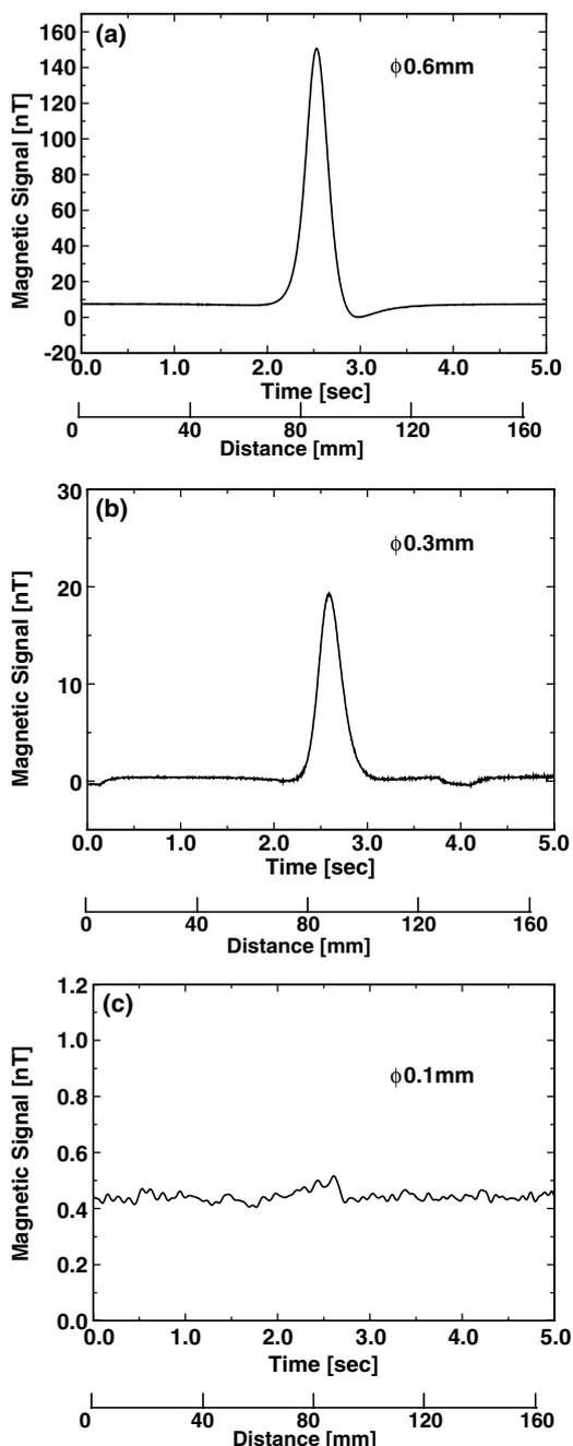
**Figure 8.** The time signal traces for the diameters (a) 0.6 mm, (b) 0.3 mm and (c) 0.1 mm of samples. For the sample of diameter 0.1 mm, a FFT filtering was applied after the data acquisition.
