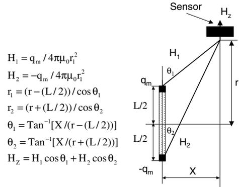
**Figure 6.** The model and the equations used for the calculation. The  $z$  component of the magnetic field intensity  $H_z$  is a function of  $r$  and  $L$ , where  $r$  is the distance from the dipole to the sensor and  $L$  is the length of the dipole.
