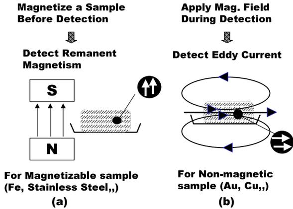
**Figure 1.** Principles of the detection system. For the non-magnetic sample case, an AC magnetic field is applied during the detection to induce an eddy current in the sample. For the magnetizable sample case, a strong magnetic field is applied to the sample prior to the detection attempt.
