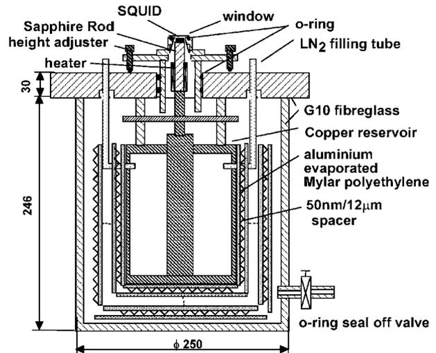
**Figure 4.** A cross-sectional view of the cryostat. This is especially designed for use with a SQUID microscope. The minimum separation between the SQUID and the sapphire window is 200  $\mu\text{m}$ .
