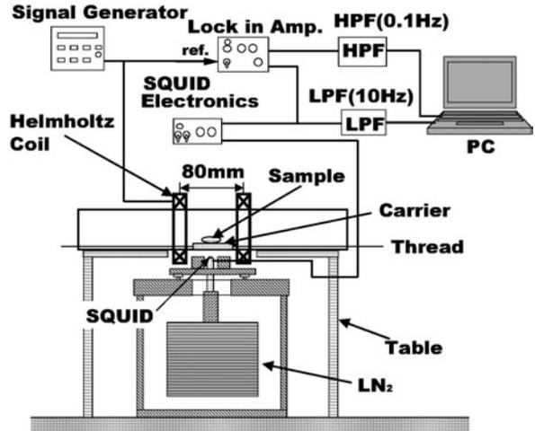
**Figure 3.** A schematic drawing of the detection system. A rectangular shaped Helmholtz coil was located above the cryostat via a table. A sample was slid onto the surface of the rectangular coil tube with constant speed.
