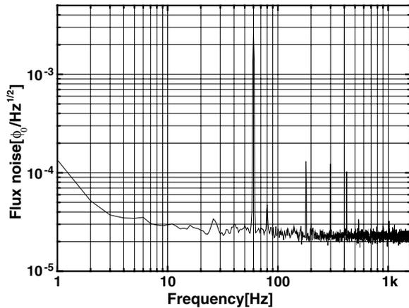
**Figure 2.** The spectral density of the flux noise of the SQUID. The magnetic flux noise in the white noise region was about  $20 \mu\phi_0 \text{ Hz}^{-1/2}$ .
