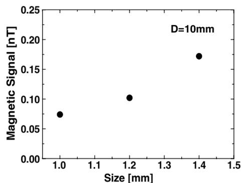
**Figure 10.** The dependence of the signal intensity on the Cu ball size. At the distance of 10 mm, the detectable minimum size for the Cu balls was 1.0 mm. The signal was proportional to the second to third power of the diameter.
