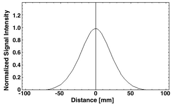
**Figure 7.** The calculated magnetic field distribution of the sample. The measured signal is asymmetric in shape, unlike the calculated signal, because of the tilt of the sample. The width of the foot of the measured signal is almost 130 mm, the same as the calculated value.
